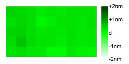
**Caption:** The Linearcoater enables super thin films of iXsenic<sup>®</sup> precursor solution with an excellent layer thickness homogeneity (range <0.5 nm)
